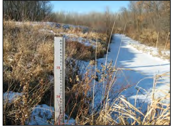
High-water staff gauge – Moose R.at Mar. Co.Hwy. #54
